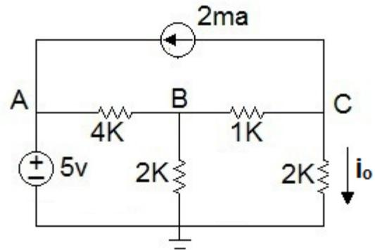
$R_{Th}$  is seen to be the 1 K resistor in series with the parallel 2K and 4K.
