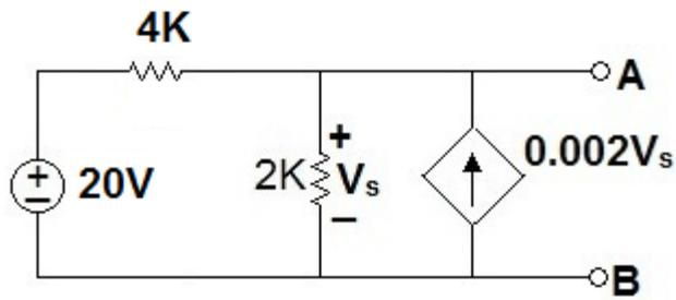
We can remedy this by placing a 1 volt source at A-B and calculating the current  $i$ .  $R_{Th} = 1/i$
