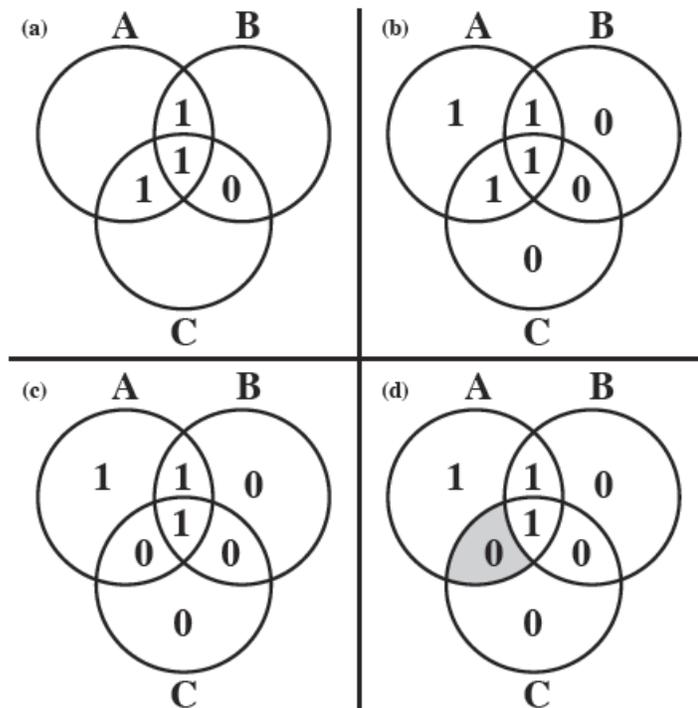
**Figure 5.8 Hamming Error-Correcting Code**
