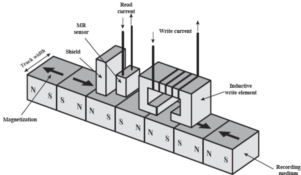
**Figure 6.1 Inductive Write/Magneto-resistive Read Head**
