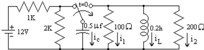
19. Write (but do not solve) the differential equation for  $V_L$  for the circuit below. Your equations should contain only  $V_L$  and  $V_g$  as variables.
