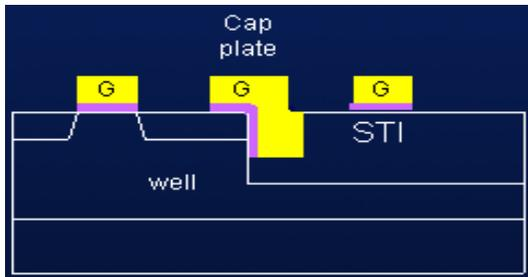
Figure 3. 1T-SRAM-Q cross-section showing vertical capacitor (FAC).
