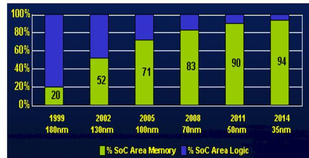
Figure 1. Increase in memory content with migration to advanced process technologies.
