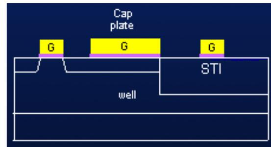
*Figure 2. 1T-SRAM cross section showing horizontal capacitor plate.*
